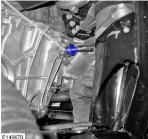
24. CAUTION: Make sure that the swarf tool is not removed by more than 15mm during this step. Failure to follow this instruction may result in damage to the vehicle. The swarf tool acts as a sealing plug, removing by more than 15mm may allow swarf fragments to enter the engine oil pan.
