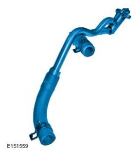
2. Identify the oil drain tube supplied in the parts kit.
