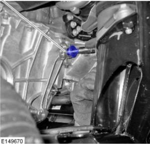
27. CAUTION: Make sure that the o-ring seal located on the oil drain tube is lubricated before installation.
